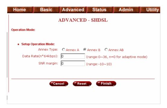
SNR margin is an index of line connection. You can see the actual SNR margin in STATUS SHDSL. The larger SNR margin, the better line connection.
