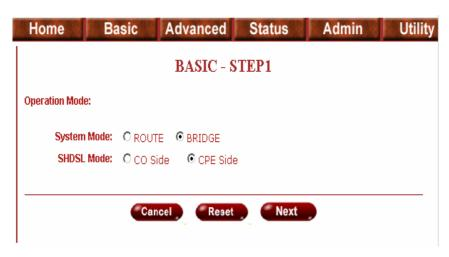
This product can be setup two SHDSL mode: CO, Central Office, and CPE, Customer Premises Equipment. For connection with DSLAM, the SHDSL mode is CPE. For LAN to LAN connection, one side must be Co and the other side must be CPE.
