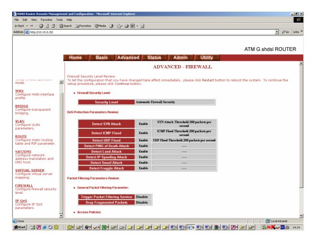
User can determine the security level for special purpose, environment, and applications by configuring the DoS protection and defining an extra packet filter with higher priority than the default SPI filter. Note that, an improper filter policy may degrade the capability of the firewall and/or even block the normal network traffic.
