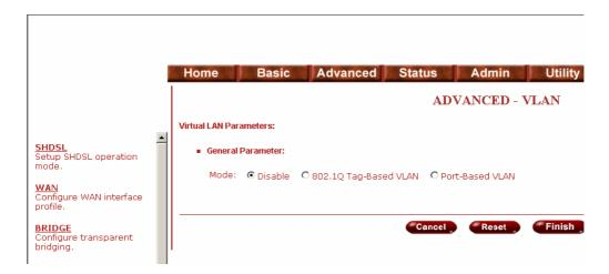
The product support two types of VLAN, 802.1Q and Port-Based. User can configure one of them to the router.
