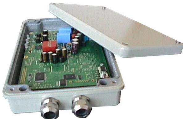
For harsh environments and outdoor use S-Access Etherlink\_II Repeaters are also available in cost effective and high profile aluminum enclosures, extending single or dual pair SHDSL (TC-PAM16/32). It offers Ethernet add/drop functionality (10/100BT, Bridge) and is protected by an IP-67 aluminum housing. The repeater can be powered locally or remotely over the DSL line. Therefore, it is configurable as power “end-point” or “pass-through”.
