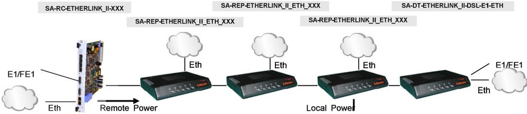
Ethernet Add/Drop Repeater Application with remote Power and local Power
