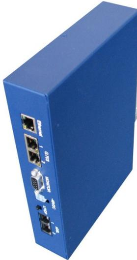
When Rail mounting is a requirement the S-Access Etherlink\_II Repeater with DIN Rail case is the right choice, extending single pair SHDSL (TC-PAM16/32) up to 5.7Mbps. It offers Ethernet add/drop functionality (10/100BT, Bridge) and comes in a blue (RAL 5003) powder coated metal housing with white labeling.
